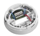
The Series 65 12V Relay Base is designed for use in both fire and security systems. For fire systems a jumper on the PCB is fitted to a 'latching' position. For security systems the jumper is moved to another position so that the base is 'non-latching'.
