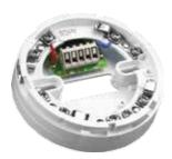
The Series 65 Standard Relay Base provides one set of volt-free, changeover (form C) contacts that change state when the detector signals an alarm.
