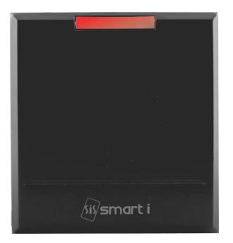
**smartRID** comes in compact 125 kHz proximity (SPR501) & 13.56 MHz Mifare<sup>®</sup> Classic smart card reader (SC504) that provides security, authentication, and access control to your entryway. This reader utilizes a Wiegand interface to provide a read range up to 3".
