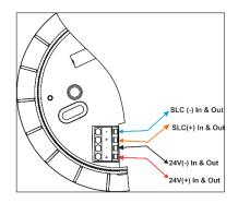
Connect the Loop Positive & Negative wires to SLC IN Terminal, observing the polarity. The wiring terminal accepts solid or stranded cables up to 2.5mm<sup>2</sup>.
