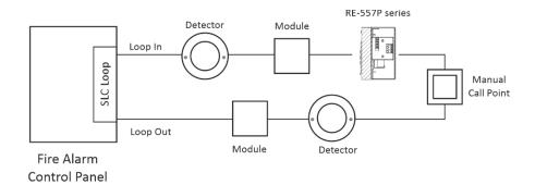
Connect the Loop Positive & Negative wires to SLC IN Terminal, observing the polarity. The wiring terminal accepts solid or stranded cables up to 2.5 mm<sup>2</sup>.
